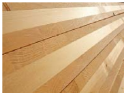
Cross Laminated Timber - CLT
