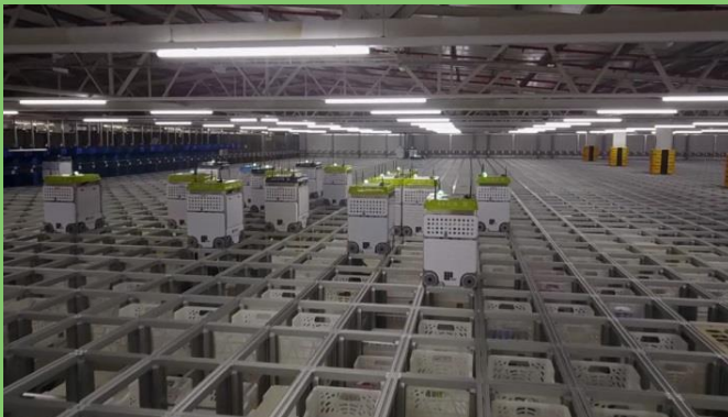
Ocado robots for grocery pick and pack...
