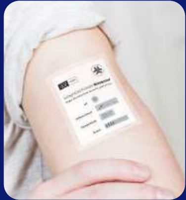
Electronic skin patches for diagnostics and monitoring
