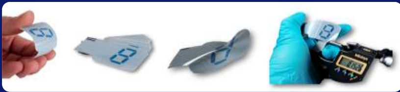
Displays printed on paper (ThinFilm)
